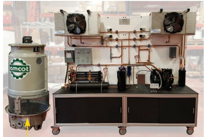
OPTIONAL WATER TOWER AND WATER PUMP
