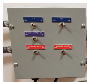
Electrical Fault Package on the back of the trainer
