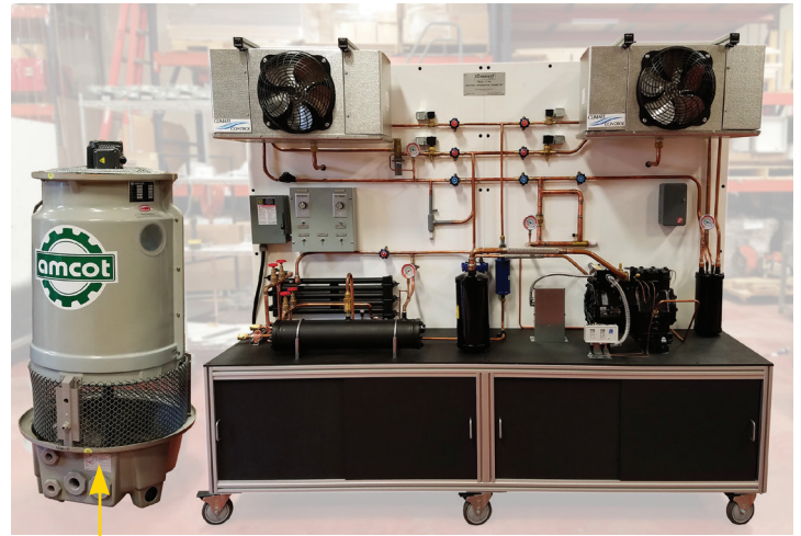
OPTIONAL WATER TOWER AND WATER PUMP
